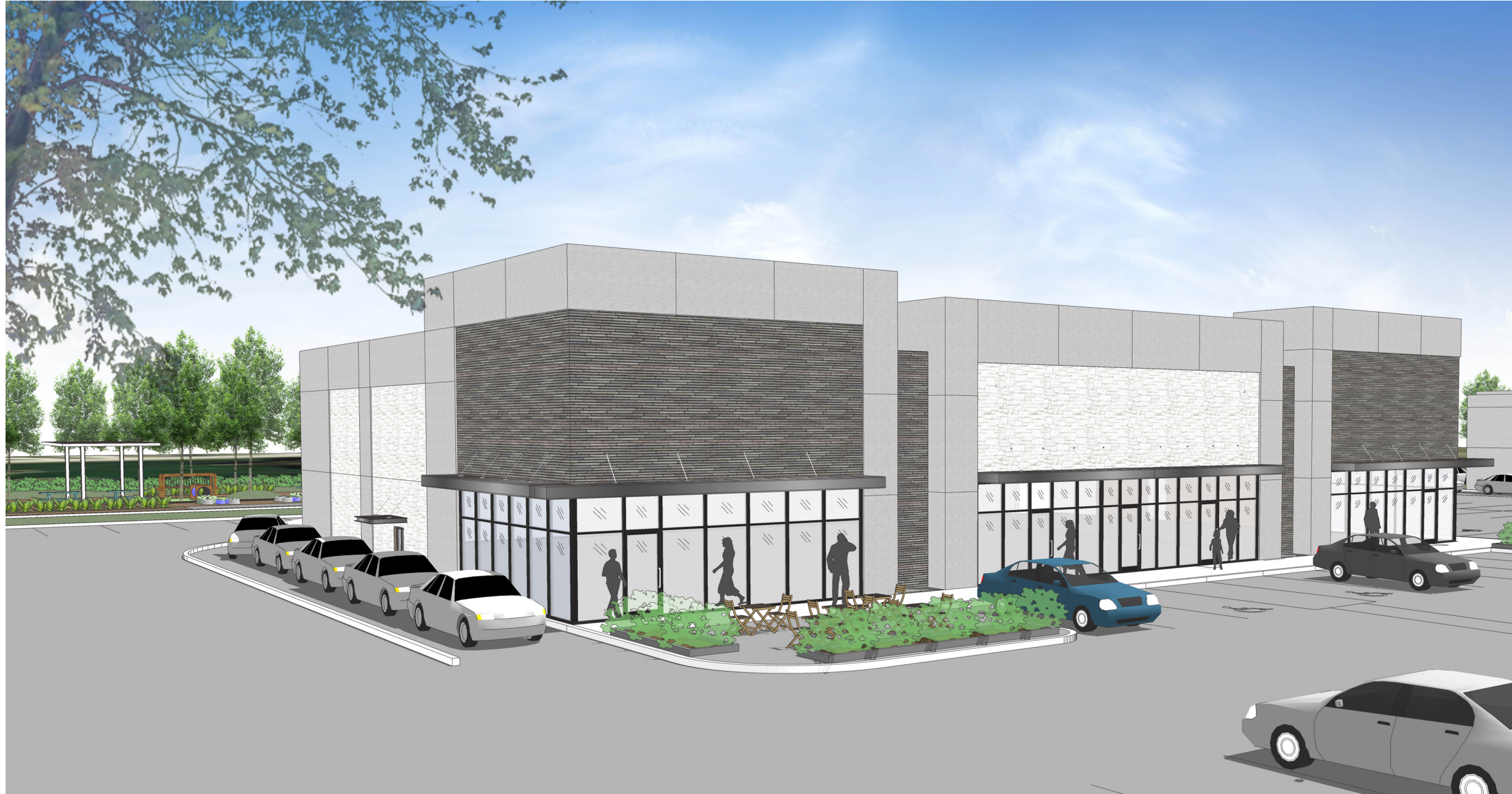
SMOOTH DIMENSIONALLY CUT 12", 8", 6" TALL BANDS OF BBCO THINSET LIMETONE VENEER - NORTHWOOD LIGHT
